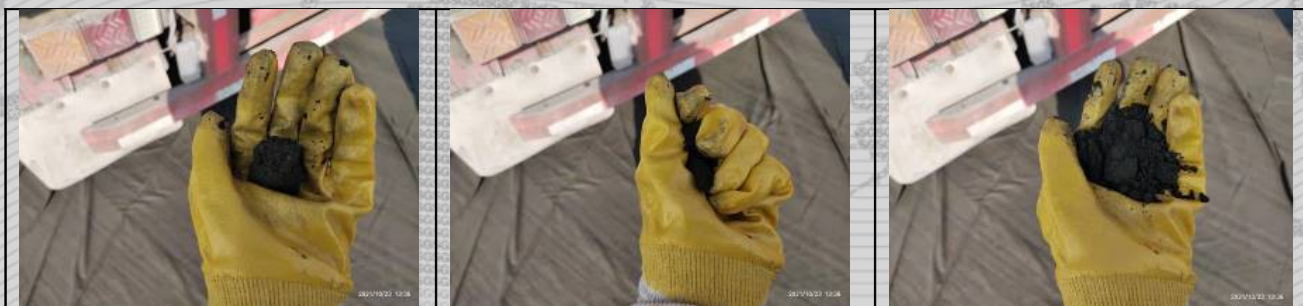
Cargo in agglomerated condition could crushed by hand pressure
